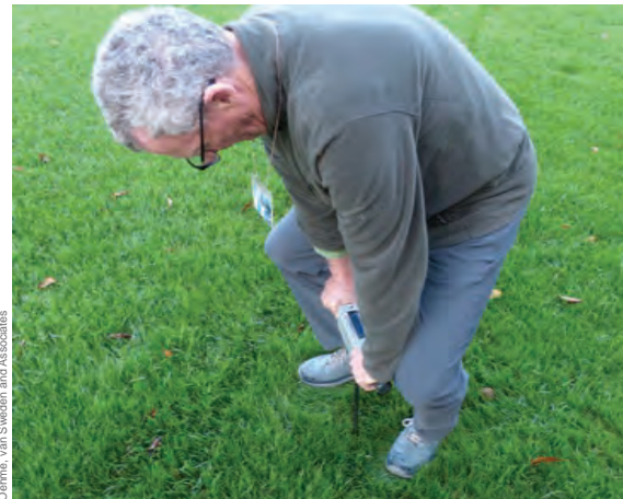
1 Penetrometer Reading by James Urban on site.
